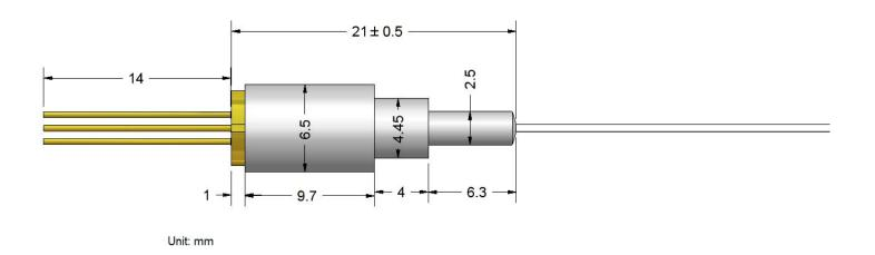
φ5.6 mm Pigtailed Coaxial Device (TO56 Header)
